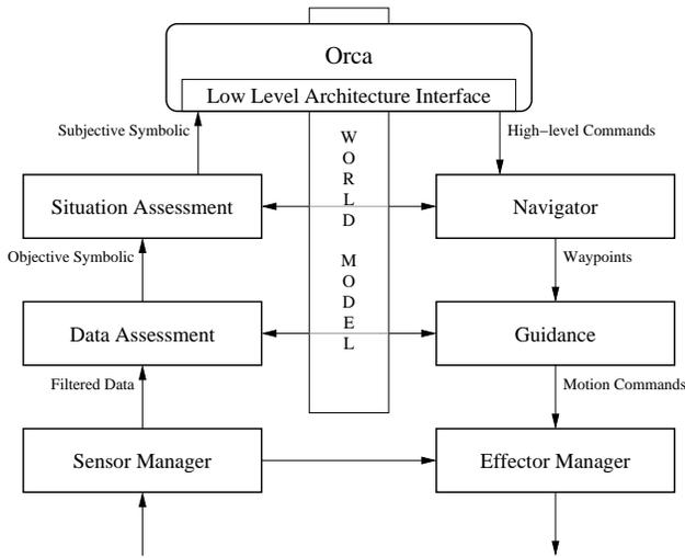
Figure 1: Orca situated in the MSEL software architecture
