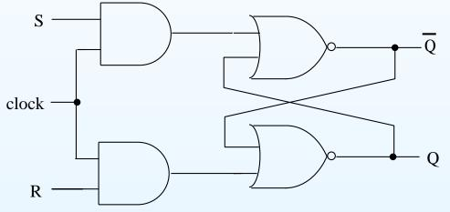
If clock is not 1, equivalent to S and R of unclocked latch being 0, and maintain state. If clock is 1, value of S and R get through AND gate.
