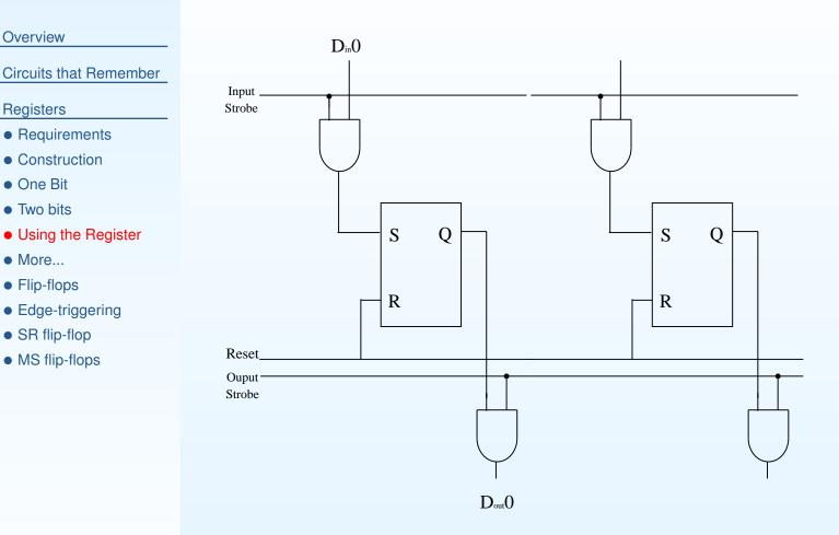
Can we just put in the data? What happens if the new data is 0, but the previous data was 1? What can we do to fix this? Need to reset each time before loading data.
