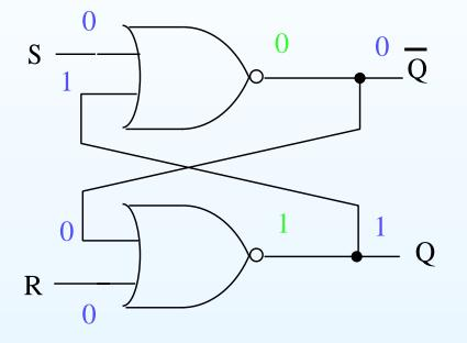
Suppose initial state is 1 and complement is 0. S and R are both 0 (neither set or reset).
