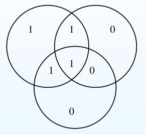
Now each bit is checked by unique combination of parity bits
