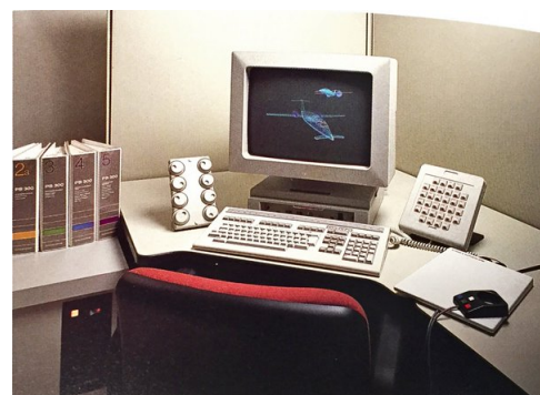
Figure 8: An Evans & Sutherland PS 300 graphics workstation. [From a tweet by @ESDigistar (Evans & Sutherland Twitter account), December 31, 2015]
