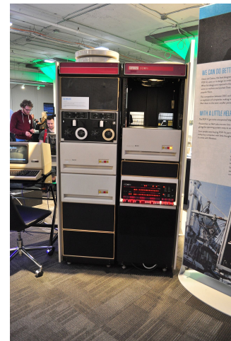
Figure 6: A PDP-11/70 minicomputer. [Joe Mabel, via Wikimedia Commons, CC-BY-SA 3.0]
