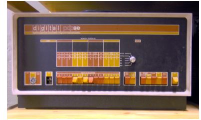
Figure 4: Front panel of a Digital Equipment Corporation PDP-8 computer, showing the toggle switches. [Photo by Arj, via Wikimedia Commons, CC BY-SA 3.0]
