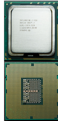
Figure 3: Front and back of an Intel Core i7 CPU. [By Atomicbre via Wikimedia Commons, CC-BY-3.0]
