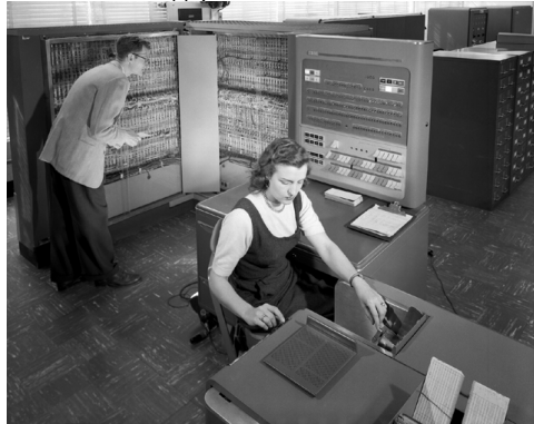
Figure 2: IBM 704 electronic data processing machine [NASA photograph].
